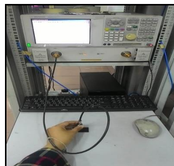
Fig. 7. Dielectric probe technique
