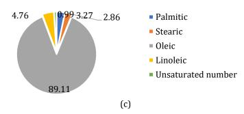
**Figure 1.** The fatty acid composition on three types of vegetable oils bio-based lubricant (a) Soybean, (b) Safflower, and (c) Sunflower [36].
