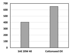
Figure 9. The wear scar comparison between SAE 20W 40 and cottonseed oil [46].
