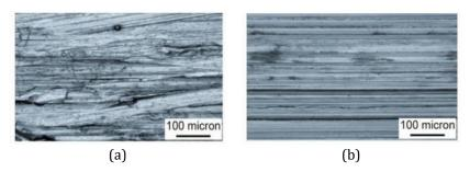
Figure 6. the wear groove at different speed of disk (a) at 0.4 m/s, (b) at 4.0 m/s [45].
