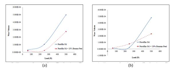
**Figure 8.** (a) wear scar diameter of paraffin oil and paraffin oil with 20% of banana peel at 500 rpm and (b) wear scar diameter of paraffin oil and paraffin oil with 20% of banana peel at 1000 rpm.
