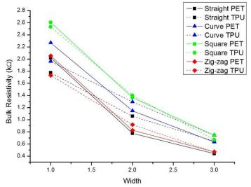
Figure 3. Bulk resistivity for test patterns with PET and TPU substrates.
