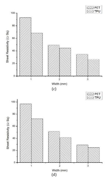
**Figure 5.** Histogram of sheet resistivity comparison for PET and TPU substrates. (a) straight pattern, (b) curve pattern, (c) square pattern and (d) zig-zag pattern.
