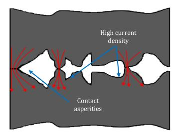
Figure 6. Diagram of constriction resistance.
