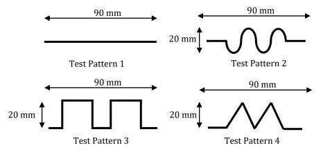
Figure 1. Conductive ink test pattern.
