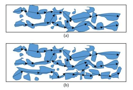
**Figure 4.** Particle distribution of the electron flow. (a) small trace width and (b) wider trace width
