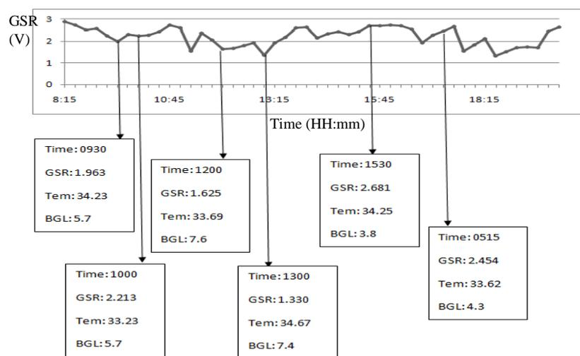
**Figure 6.** GSR graph with the respective blood glucose level for User 1.
