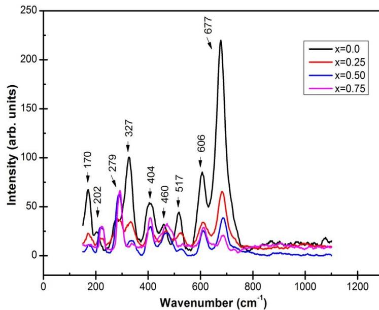
**Figure 3.** Raman spectra for  $\text{Sr}_{1-x}\text{Co}_x\text{Fe}_{12}\text{O}_{19}$  hexaferrite ( $x=0.0, 0.25, 0.50$  and  $0.75$ ) at room temperature.
