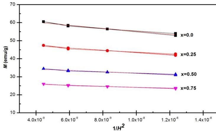
**Figure 5.** Magnetization ( $M$ ) against  $1/H^2$  plots for  $Sr_{1-x}Co_xFe_{12}O_{19}$  hexaferrite ( $x=0.0, 0.25, 0.50$  and  $0.75$ ).
