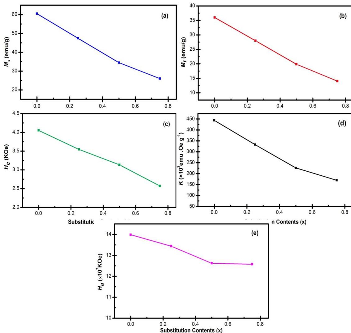
**Figure 6.** (a) Variation of saturation magnetization ( $M_s$ ), (b) remanence ( $M_r$ ), (c) coercive field ( $H_c$ ), (d) effective anisotropy constant ( $K_{eff}$ ) and (e) anisotropy field ( $H_a$ ) as a function of substitution contents (x) for  $Sr_{1-x}Co_xFe_{12}O_{19}$  hexaferrite.
