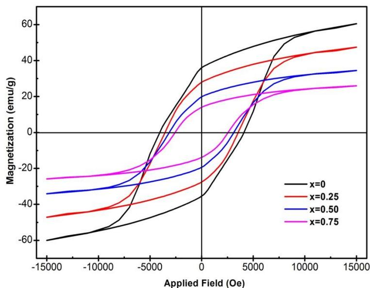
**Figure 4.** The applied-field dependence of the magnetization hysteresis loops of  $\text{Sr}_{1-x}\text{Co}_x\text{Fe}_{12}\text{O}_{19}$  hexaferrite ( $x=0.0, 0.25, 0.50$  and  $0.75$ ) at room temperature.
