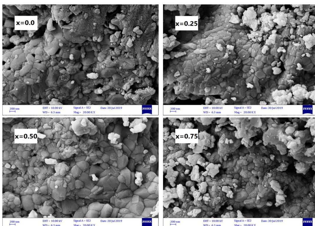
**Figure 2.** FE-SEM images of  $\text{Sr}_{1-x}\text{Co}_x\text{Fe}_{12}\text{O}_{19}$  hexaferrite ( $x=0.0, 0.25, 0.50$  and  $0.75$ ).
