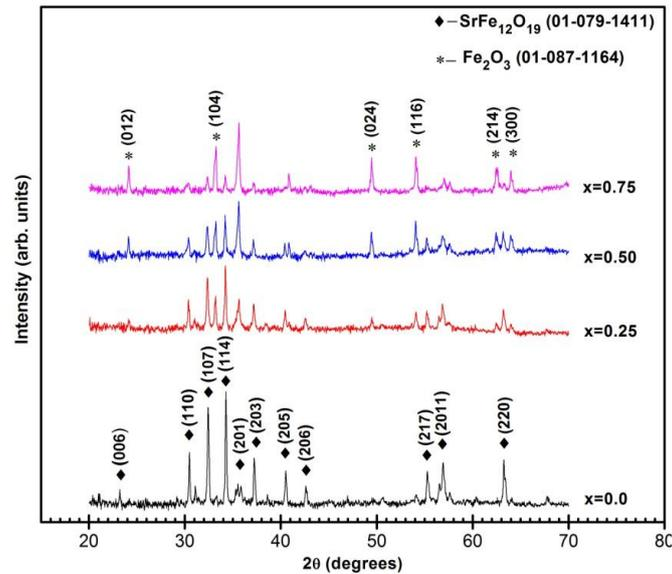
**Figure 1.** XRD pattern of  $\text{Sr}_{1-x}\text{Co}_x\text{Fe}_{12}\text{O}_{19}$  hexaferrite ( $x=0.0, 0.25, 0.50$  and  $0.75$ ) at room-temperature.
