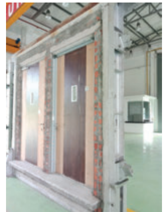
Installed fire doors are tested using the Fire Testing Furnace. This set-up is then mounted to the front of the Fire Testing Furnace to stimulate an actual site installation.
