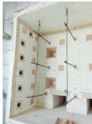
Fire Testing Furnace showing the heat probes along the vertical and horizontal planes. On the side is the heat source using gas. The back section is the vision panel while the bottom is the exhaust of the furnace.
