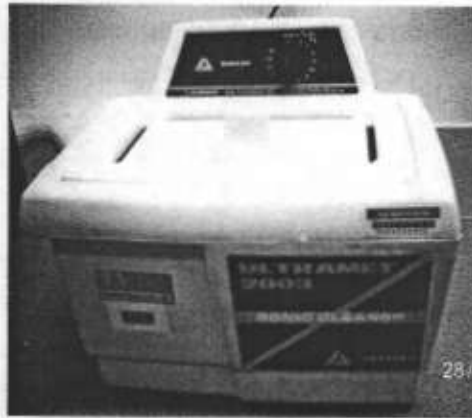
Figure 5b : Buehler Ultramet 2003 sonic cleaner
