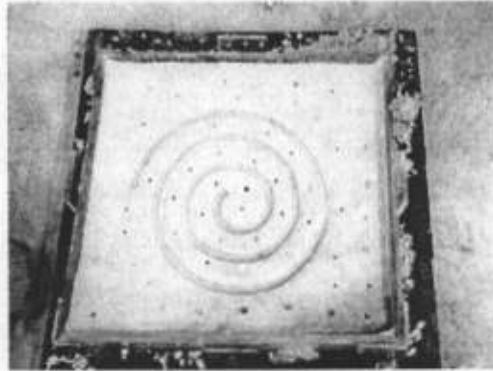
Figure 10: spiral pattern for flowability test
