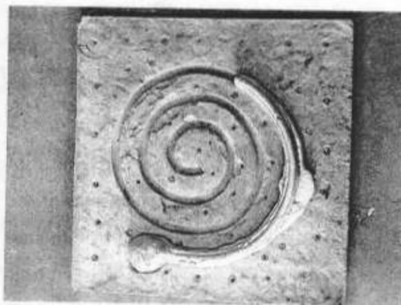
Figure 11c: The cast spiral open mould and a result of flowability test
