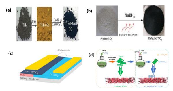
**Figure 2.** Schematic diagram of : (a) synthesis of Ti<sup>3+</sup> self-doped rutile TiO<sub>2</sub> using oxidation process [33]. (b) synthesis of Ti<sup>3+</sup> self-doped TiO<sub>2</sub> using reduction agent[42]. (c) synthesis of p-type TiO<sub>2</sub> using atomic layer deposition[43]. (d) formatiom of TiO<sub>2</sub> p-n homo-junction using in-situ decorating n-type TiO<sub>2</sub> QDs on p-type TiO<sub>2</sub> sheets[20].
