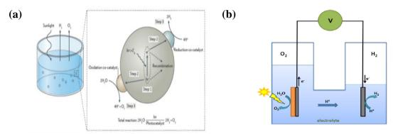
**Figure 7.** Photocatalytic water-splitting reactions: (a) photo-chemical reaction [62]. (b) photoelectrochemical reaction [59].
