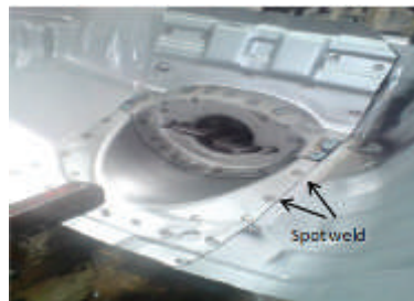
Figure 1: (b) Spot weld on automotive part.
