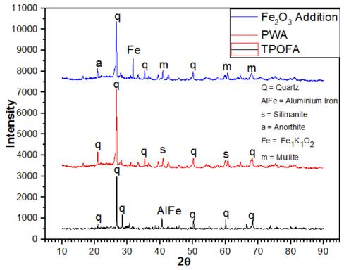
Figure 2. XRD pattern of treated POFA (TPOFA), porcelain without the addition of  $Fe_2O_3$  (PWA) and porcelain with the addition of  $Fe_2O_3$ .
