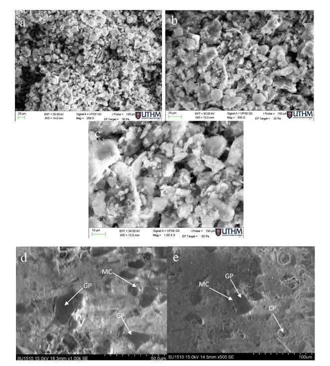
**Figure 1.** SEM of POFA powder (a,b and c) and porcelain without addition of ferum  $Fe_2O_3$  (d) and after addition (e). [MC = micro crack, CP = closed porosity, GP = Glassy phase] (d) and after addition (e). [MC = micro crack, CP = closed porosity, GP = Glassy phase].
