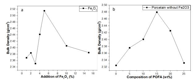
Figure 4. The bulk density of porcelain with and without the addition of Fe<sub>2</sub>O<sub>3</sub>.
