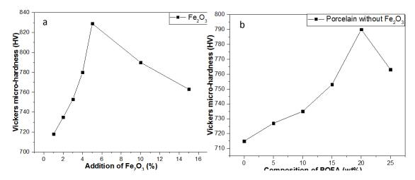
Figure 5. Vickers microhardness of Porcelain made with and without the addition of Fe<sub>2</sub>O<sub>3</sub>.
