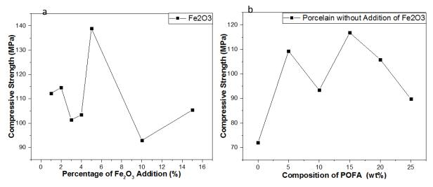
Figure 3. The compressive strength of porcelain with and without the addition of Fe<sub>2</sub>O<sub>3</sub>.
