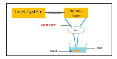
Figure 1. The essential features of Nd-YAG laser.
