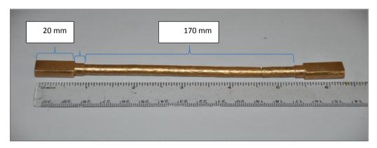
Figure 2. Metal Sample after torsion testing.
