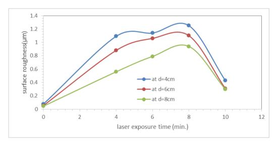
**Figure 5.** Surface roughness versus laser exposure time for 4 cm, 6cm and 8 cm distances from laser source.
