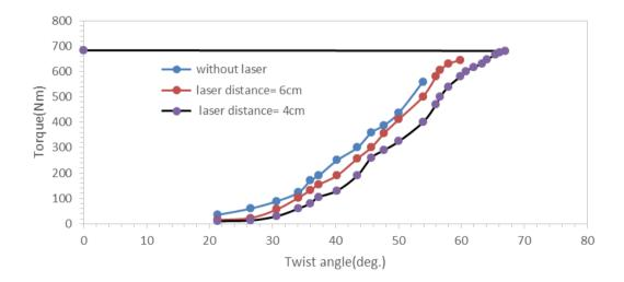
**Figure 3.** Torque force as a function of twist angle of 8 minutes exposure time with and without laser treatment.
