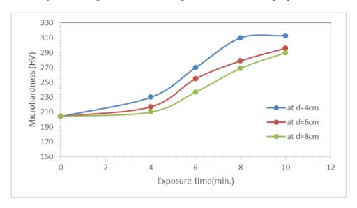
**Figure 6**. Micro hardness versus laser exposure time of 4 cm, 6 cm and 8 cm of distance from laser source.
