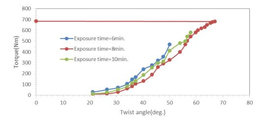
**Figure 4.** This curve compare between the Torque forces as a function of twist angle of 4 cm distance from the laser source with 8 minutes exposure time.
