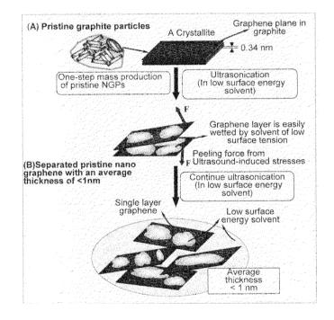
Figure 16. The essential procedures used to produce single-layer or few-layer [160] [161].
