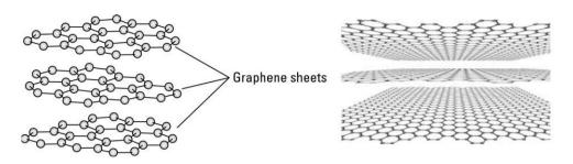
Figure 8. Graphene sheets that exfoliated from graphite [32].
