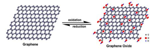
Figure 13. Scheme of structural model of graphene and graphene oxide (GO) [73-74].
