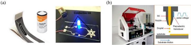
Figure 15. (a) conductive ink. (b) Inkjet printing technology [154] [155].
