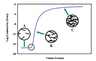
Figure 4: The dependence of electrical Conductivity on the filler content [25].
