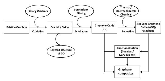
Figure 14. Schematic representation of the graphene functionalization [72-75].
