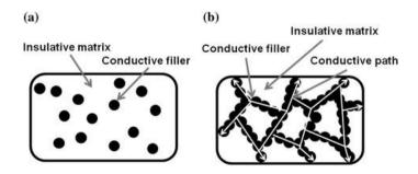
**Figure 3**. Filler distribution in polymer composite: (a) at low content, (b) conductive path at high enough content [24].
