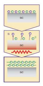
Figure 11. Schematic illustration of the epitaxial growth of graphene on SiC method [49].
