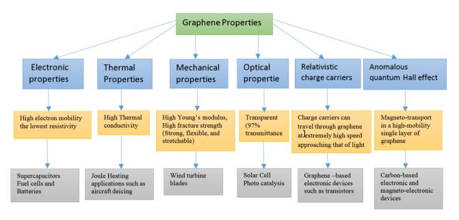
Figure 9. Graphene properties and applications [31-33].
