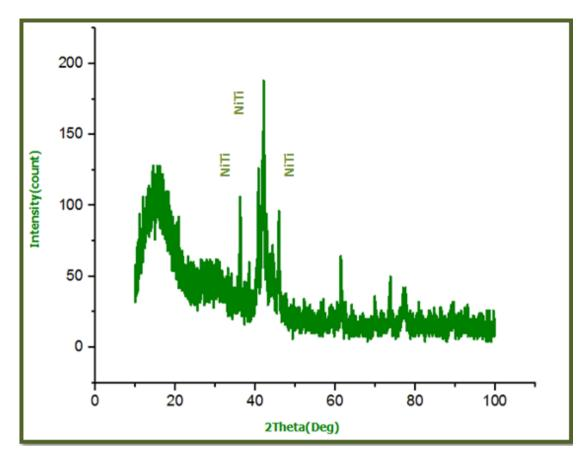
From Table 5 the average value of the crystalline size was found to be equal to 16nm.
