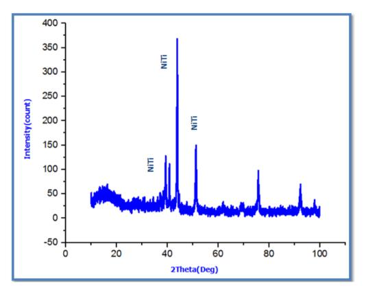
Figure 4. XRD result of the sample after irradiated with 300mJ of laser energy.
