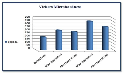
Figure 12. Hardness profile before and after irradiated samples with different laser energies.
