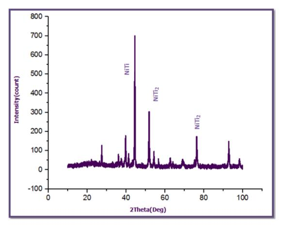
Figure 6. XRD result of the sample after irradiated with 500 mJ of laser energy.
