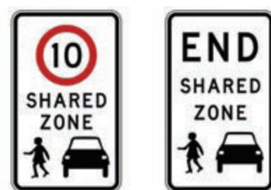
Figure 4: Entry and exit signages for shared space zones
