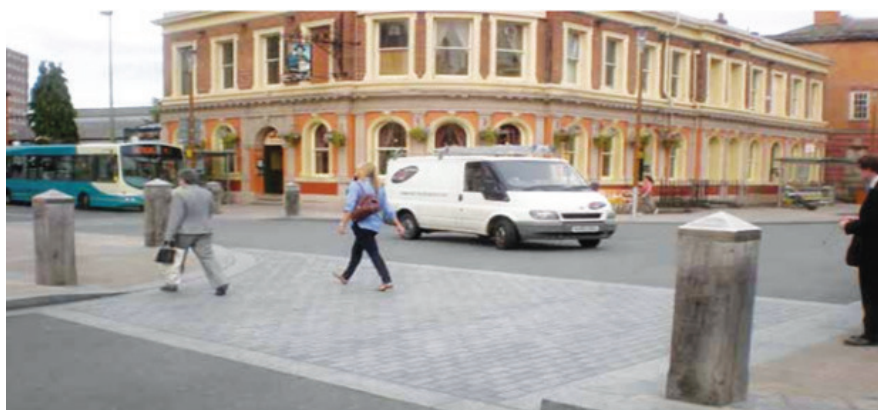
Figure 2: Courtesy crossing (Source: Department for Transport, UK, 2011)
