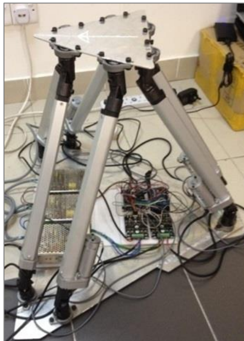
Figure 1: Prototype of Stewart platform for track cycling simulator
