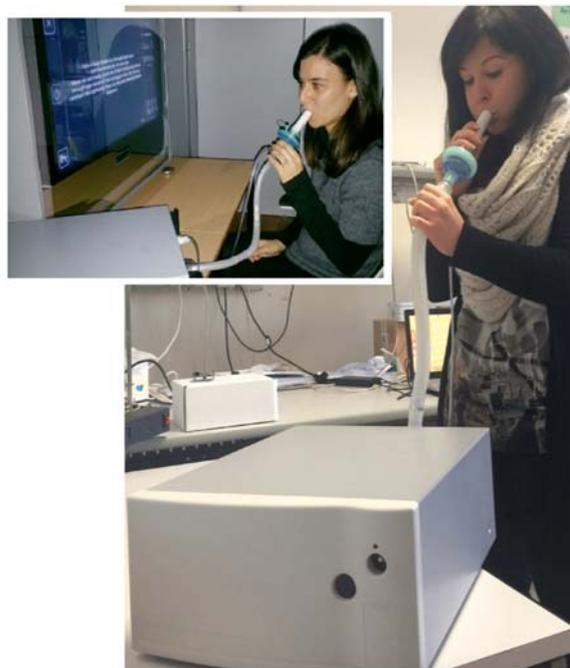
**Fig. 2.** The two Wize Sniffer's operation modes: as a Wize Mirror’s tool (on the left) and as a stand-alone device (on the right).
