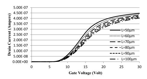
Figure 7: Variation of drain current as a function of gate voltage for different values of channel length
