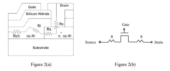
Figure 2: (a) Parasitic resistance (R) components of the n-channel top gated nc-Si TFT and (b) Equivalent circuit of the TFTs used for device simulation
