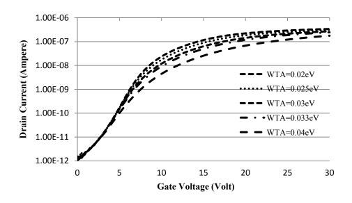
Figure 5: Variation of drain current as a function of gate voltage for different values of tail states
