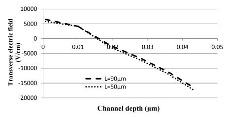
Figure 8: Channel length dependence on Transverse electric field
