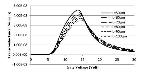
Figure 6: Variation of transconductance as a function of gate voltage for different values of channel length
