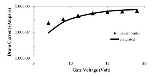
Figure 10: Plot of the transfer characteristic of nc-Si top-gated TFT (W=200 $\mu$ m and L=50 $\mu$ m) simulated at V<sub>DS</sub>=10V for WTA=0.02 and R=10<sup>6</sup>  $\Omega$ . Solid line shows the experimental results of C.H.Lee et. al. [30] and dotted line shows simulated results
