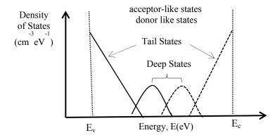
Figure 1: Density of states within the band gap of nc-Si
