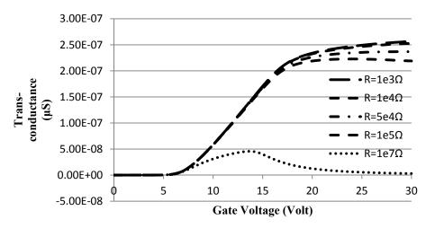
Figure 9: Variation of transconductance as a function of gate voltage for different values of parasitic resistance
