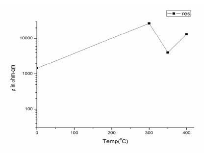
Fig. 6: Tem. (  ${}^\circ\!\!C$  ) Vs. Resistivity of TiO\_2 and Mg\_{0.01}Ti\_{0.99}O\_2 thin film annealed at different temperatures
