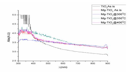
Fig. 3: Absorption spectra of  $TiO_2$  and  $Mg_{0.01}Ti_{0.99}O_2$  thin film annealed at different temperatures
