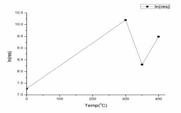
Fig. 5: Tem. (°C ) Vs. ln(Res.) of TiO<sub>2</sub> and  $Mg_{0.01}Ti_{0.99}O_2$  thin film annealed at different temperatures
