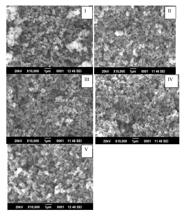
Fig. 7: SEM micrographs of (I) TiO<sub>2</sub> As-Is,(II) Mg doped TiO<sub>2</sub> As-Is,(III) Mg doped TiO<sub>2</sub> annealed at 300 °C, (IV) Mg doped TiO<sub>2</sub> annealed at 350 °C, and (V) Mg doped TiO<sub>2</sub> annealed at 400 °C.
