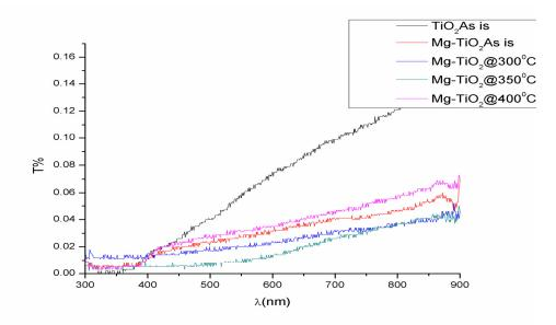
Fig. 2: Transmitted spectra of TiO<sub>2</sub> and Mg<sub>0.01</sub>Ti<sub>0.99</sub>O<sub>2</sub> thin film annealed at different temperatures
