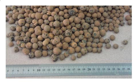
Figure 3.7: Batch 2 LWA of 8-16 mm.
