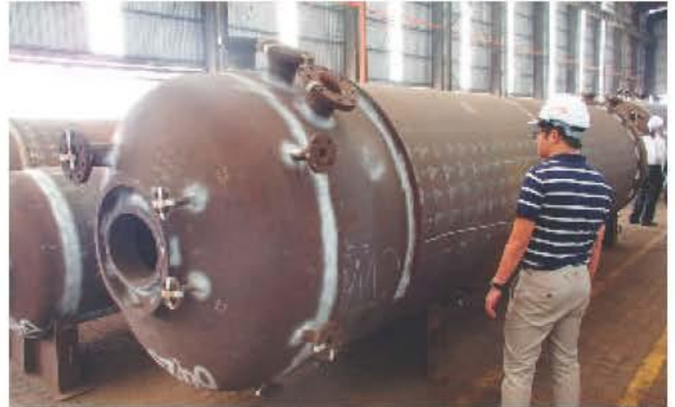
Factory visit: A steam drum with completed marking and radiography test on shell and dish heads. Ready for drilling on different nominal sizes of tubes.
