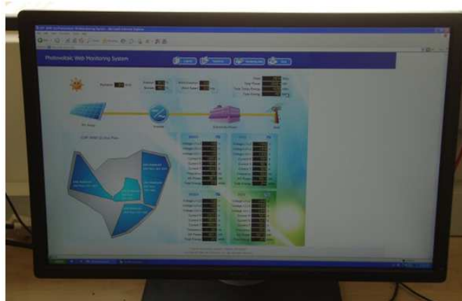
Fig. 3. SCADA system used for monitoring and recording purposes
