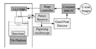
Figure 2 A block diagram of C-Scan Imaging setup [7]
