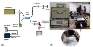
Figure 9 Swept Source Optical Coherence Tomography (SS-OCT) system; (a) Schematic diagram of SS-OCT, (b) Real SS-OCT system [19]
