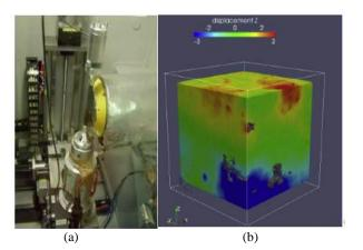
Figure 7 (a) Experiment setup for inspection system (b) 3D tomogram of aluminium alloys with pores [14]
