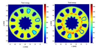
Figure 5 Complete C-scan of a defect free sample (left) and a defected sample (right) [12]
