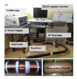
Figure 3 Photographs of the experimental set up, showing: (a) a view of the whole experimental apparatus; (b) coil arrangement in the MsS sensor used for the experimental study and (c) MsS Sensor [11]
