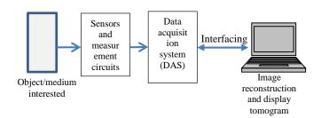
Figure 1 Basic block diagram of tomography system
