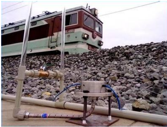
Fig. 4. FBG settlement sensor application.
