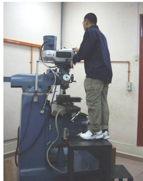
Fig.5. Poor methods for maintenance
