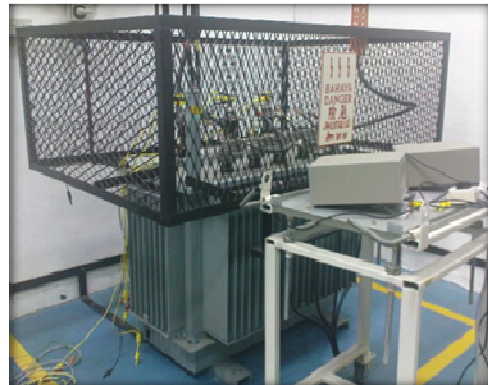
Fig. 8. A sample of an appropriate machine guarding
