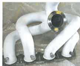
Ceramic coating on automotive part
