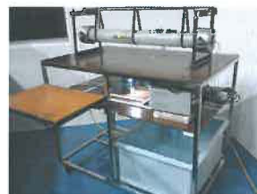
Automated UEWS pressure test rig setup
