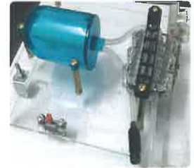
Full Set of Connection of PEM Fuel with H2 Storage Tank
