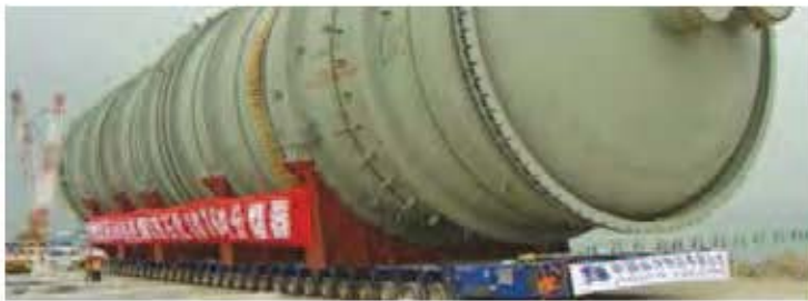
Figure 3: Example of similar oversized cargo using the Gold holder 24 lines trailer
