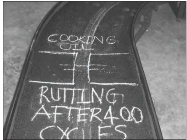
Figure 18: Rutting after 400 cycles at ACW14 exposed to cooking oil
