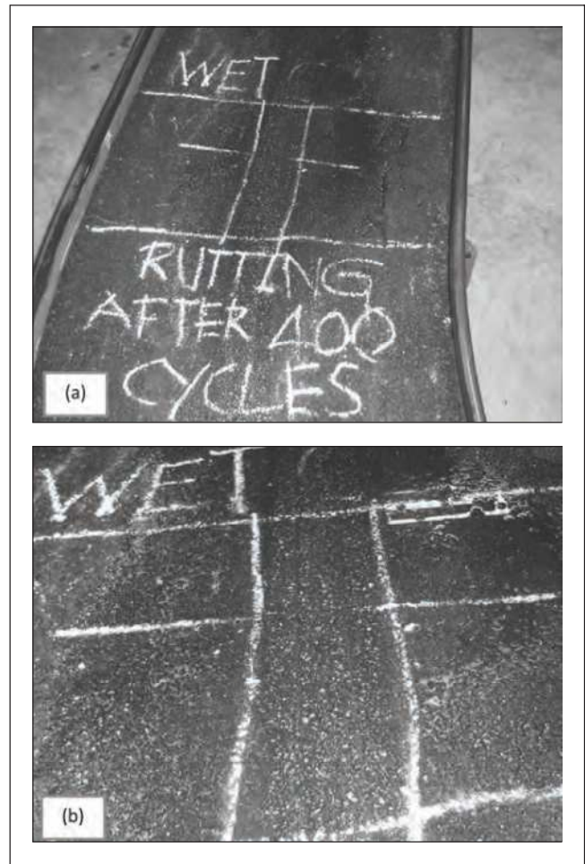
Figure 13: Stripping of aggregates occurred after 400 cycles when ACW14 was exposed to continuous wet conditions
