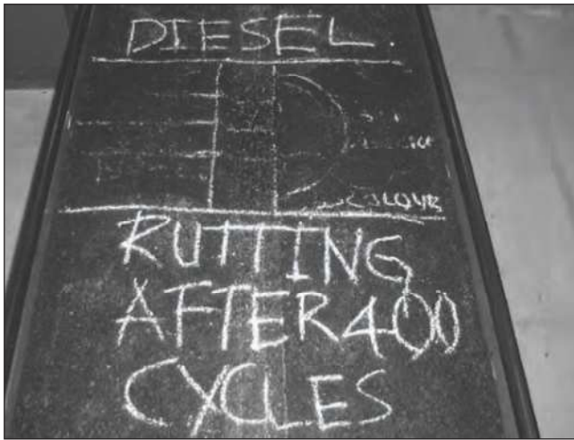
Figure 17: Rutting after 400 cycles at ACW14 exposed to diesel
