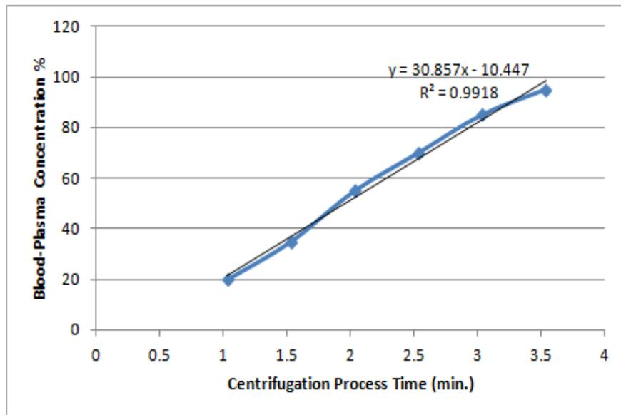
Figure 5. Blood-plasma concentration versus centrifugation time.
