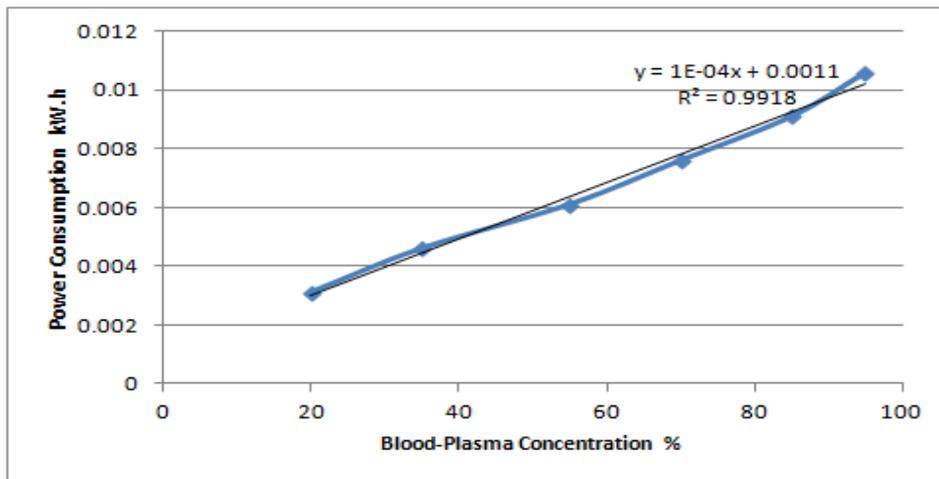
Figure 7. Centrifuge device power consumption measurements for (20-100)% Blood-plasma concentration.
