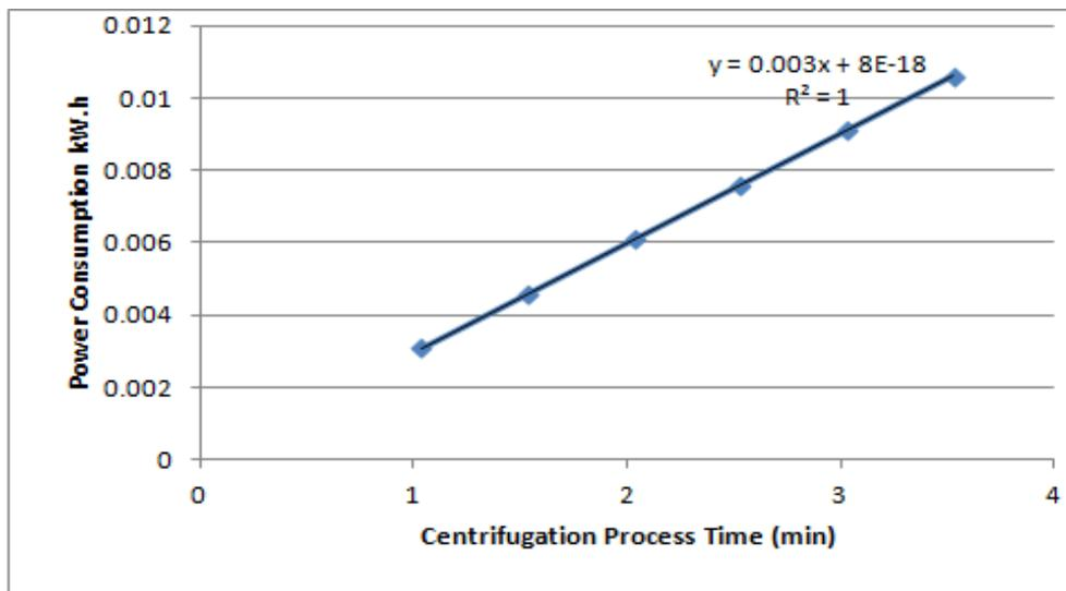
Figure 6. Power consumption versus 1ml blood sample centrifugation time.
