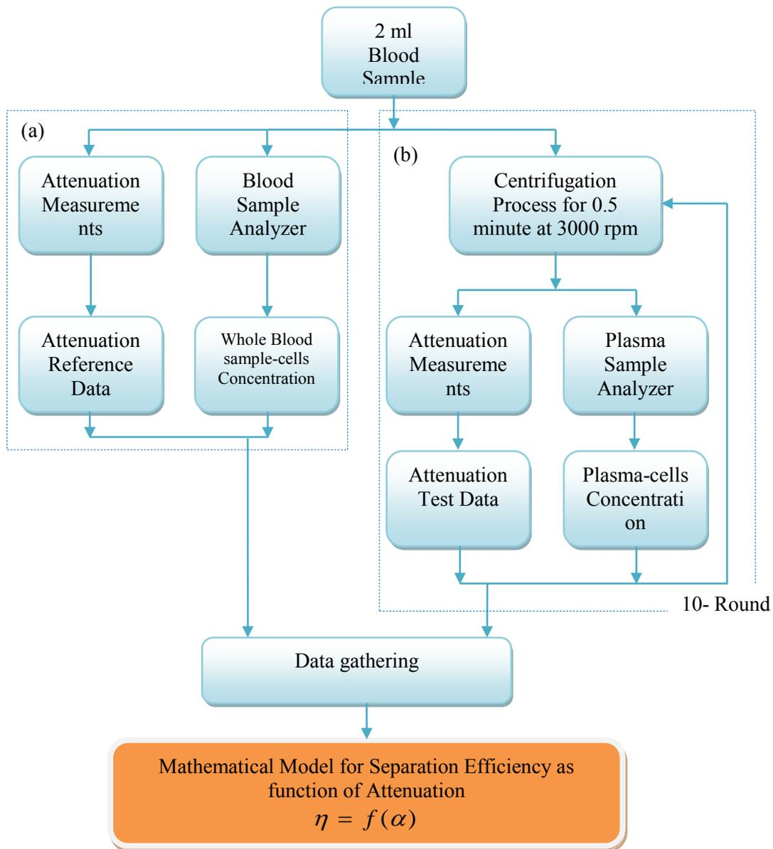
Fig.4. Experimental procedure sequence for one blood sample test.
