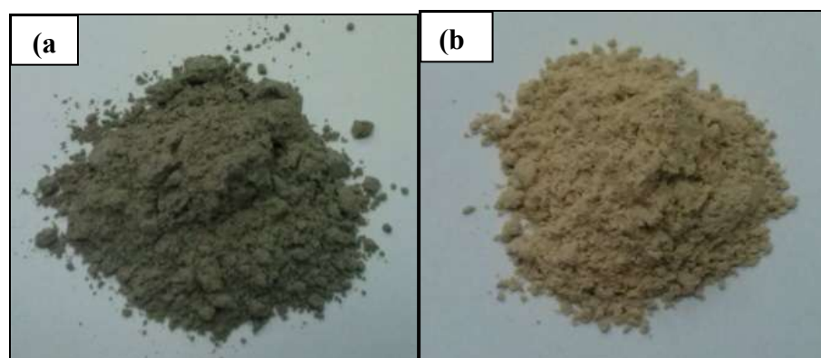
Fig. 4: Digital photo of palm ash (a) before (b) after citric acid leaching treatment.
