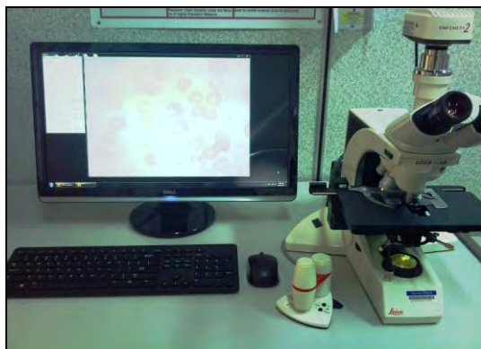
Fig.1 A set of Leica DLMA microscope, Infinity-2 digital camera and personal computer interfaced together to acquire the malaria images
