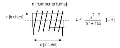
Figure 2.1: Calculations of inductor value
