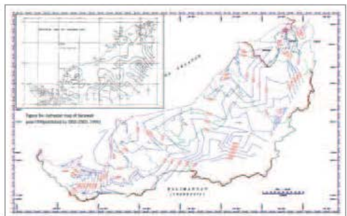
Figure 9: Generated isohyetal map of Sarawak year 1990 with interval of 360 mm by Autocad Civil 3D
