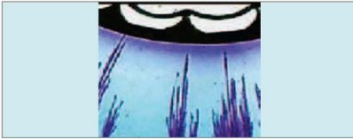
Figure 1: Typical Water Tree in Power Cables
