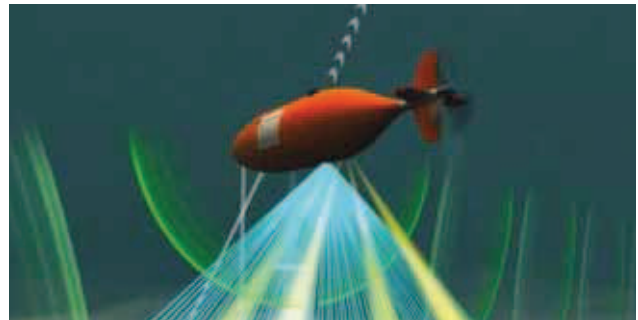
Figure 1: Sidescan sonar survey by UUV
