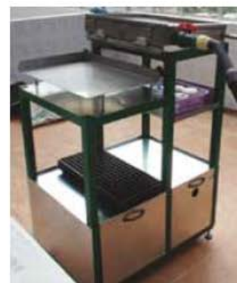
Figure 3: Mechanical seed dispensing machine
