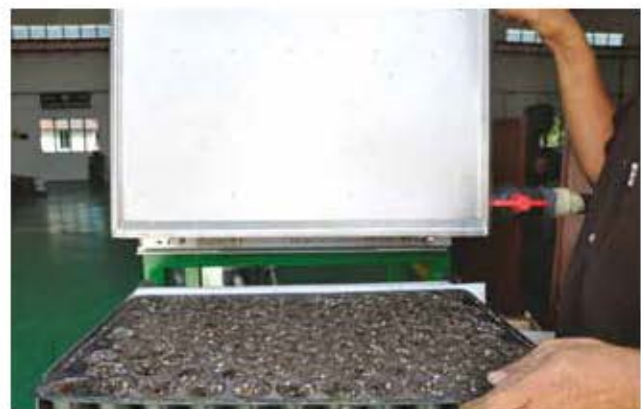
Figure 6: Dispense plate is holding seed at each perforation before the receptacle turn 180 degree facing the nursery tray to release seed into the cells
