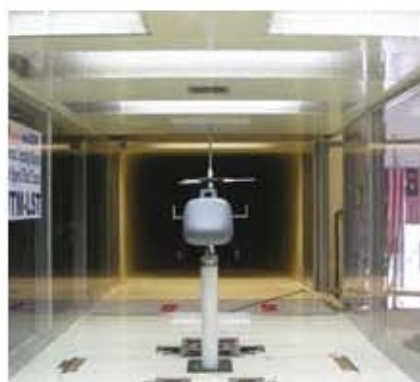
Figure 2: Model with short blade during testing at UTM-LST (looking downstream)
