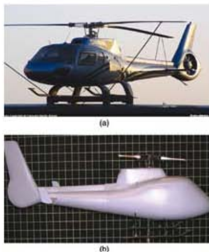
Figure 1 (a) Eurocopter 350Z Helicopter Prototype (b) A generic 350Z model with 1:7.126 scaled-down
