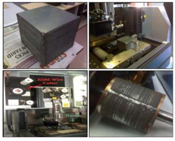
Fig. 2: Copper Rotor Fabrication Procedures.
