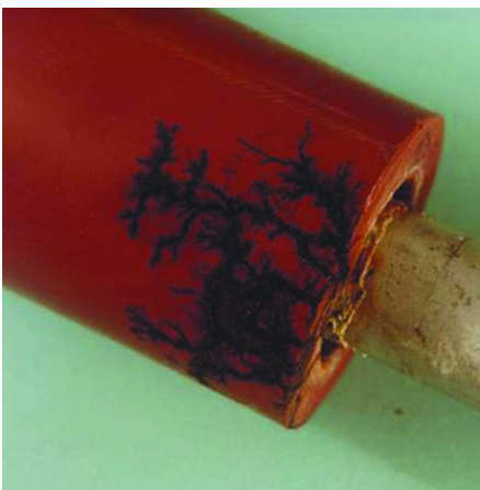
Signs of PD tracking on a HV cable insulation
