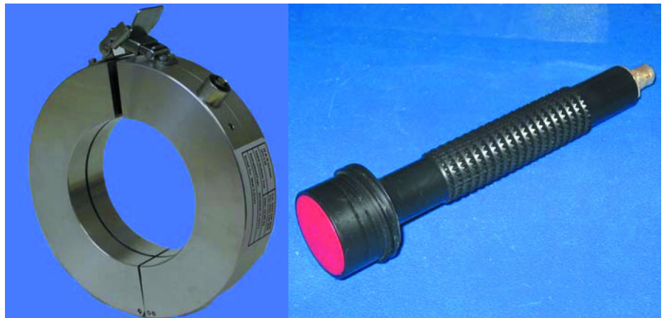
A HFCT and a TEV detector used in the demonstration
