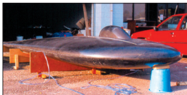
The body shell of "SURIA KAR 2" is fabricated from carbon composite material
