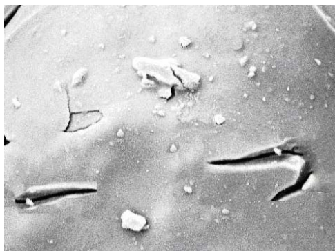
Fig. 2: Scanning electron micrographs of TiO 2 thin film immobilized on quartz sand. Conditions: calcinations temperature = 600°C. Magnification of 1500 X
