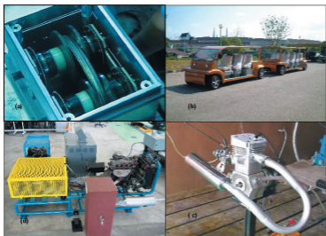
Figure 1: Research products (clockwise from top left): (a) manually-operated CVT, (b) people's mover: the Tramcar, (c) two-stroke air-cooled engine, and (d) parallel-electric hybrid powerplant for automotive applications.
