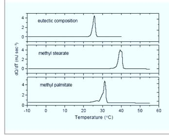
*Figure 1: The endothermic DSC thermograms of: (a) methyl palmitate (b) methyl stearate and (c) their eutectic mixture [19].*
