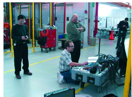
Figure 5: Voltage sag immunity testing
