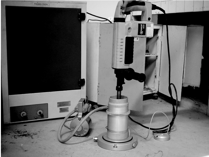
Figure 3: Compaction of samples using vibratory hammer
