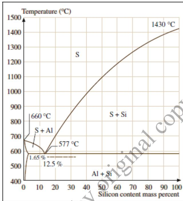
Figure 2.2 : Phase diagram of Al-Si alloy system (Martienssen, 2005)
