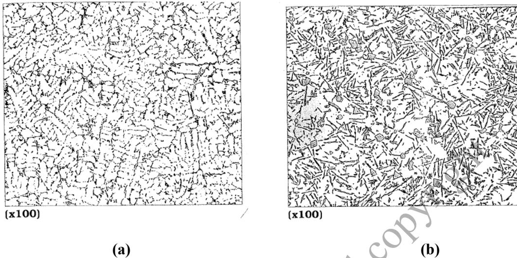
Figure 2.3 : Microstructure of Al-Si alloy; (a) hypoeutectic alloy, and
