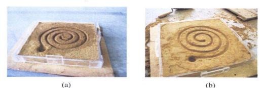
Figure 1 : Flowability mold. (a) Sand molding mold, (b) Green sand molding mold.
