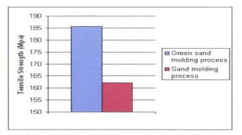
Graph 2: Graph tensile strength of send and green sand molding process
