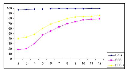
Figure 2: Effect of pH on methylene blue adsorption (dye concentration of 250 mg/L, adsorbent dosage= 0.4 g/ L and contact time = 2 hours.)
